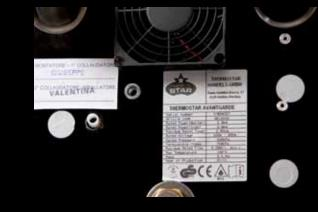
Before using your Thermostar, please ensure that there is no visible damage to the appliance. Verify that the volt and ampere ratings for your power source match those listed on the appliance sticker.
